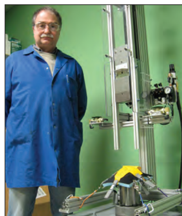
IMPACT ARMOR BEING TESTED AT AEROSTICH R&D.
