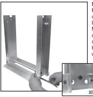
Step 2. Attaching the Base. Attach each Base (a) to the bottoms of the Sidearms using a 1" Roundhead Bolt (k) and a Locking Nut (n). There are two per side. Make sure the bolt heads are facing outside and the nuts are facing inside, as shown (detail 1). The Sidearms have been specially machined to fit this exact way. Tighten with 5mm Allen wrench and
