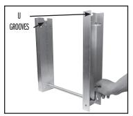
Step 1. Stabilizer Bar and Sidearms. Attach each end of the Stabilizer Bar (c) to the two Sidearms (b) using a 3/4" roundhead bolt (I) and lock washer (o) for each end of the stabilizer, as shown. Make sure that the "U Groove" in each Sidearm is at the top. Also, make sure that each Sidearm is facing as shown in the photograph. Tighten with 5mm Allen wrench.
