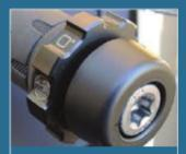
Bar end lock with oversize knurled end to help make adjusting on-and-off easier.
