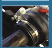
Universal Vista Cruise type owner-adapted to BMW R1200R. Owner modifications include: 1.) Throttle housing cover modified to provide stationary attachment point via custom steel plate, flush set-screws and JB Weld epoxy. 2.) Friction adjustment screw modified to be adjustable without tools. 3.) Twist grip inner flange modified/partly removed to allow inner friction ring to be installed.
