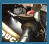
NEP brand thumb flip friction lever owner-adapted to Ducati Multistrada. Owner modifications include: 1.) stationary end held with zip tie, 2.) friction adjustment screw replaced with custom made oversize aluminum knob, 3.) inner friction surface circumference filed/sanded/enlarged to exactly match throttle housing diameter.
