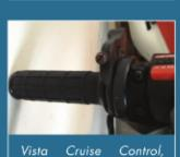
owner adapted to Honda XR650L. Owner modifications include: 1.) Stationary side of clamp held to throttle housing with small set screw via owner-tapped threaded hole. 2.) Friction screw pressure adjuster modified to be adjustable without tools.
