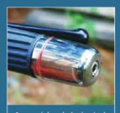
Bar end throttle lock which requires rotating hand and heel of palm several times to add frictional resistance. Simple bolt-on installation, though not the easiest to 'off-on' actuate.
