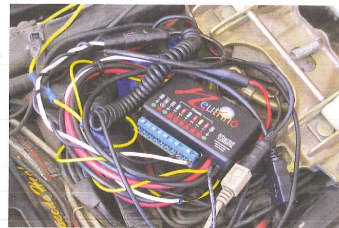
(Fig. 3) The black box takes up very little space under the seat.
